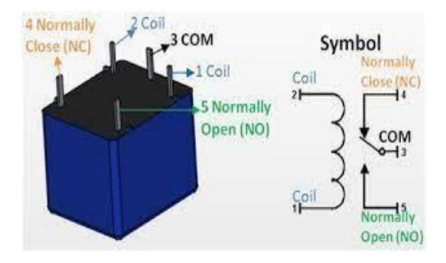
Relaysarenothingbutmechanicalswitchesoperatedusingelectromagnetic inductiontechnique.Whenyougive DC supply to 2 of its terminals ofelectromagnet, switch is shifted from N/C
