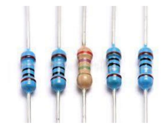
Α resistor is passive two-terminal a electric al component that implements electric al resistance as a circuitelement. In electronic circuits, resistorsare used to reduce current flow, signallevels, voltages, bias adjust to divide active elements, and terminate transmission lines, among other uses.
