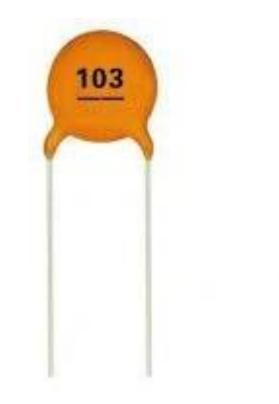
This is a 0.01uF -(103)Ceramic CapacitorUse thiscapacitorforpowerdecoupling, having asmooth powerinyour circuit, timingcircuits et alwaysagood ideatoput oneofthese ne powerpinsof amicrocontroller.
