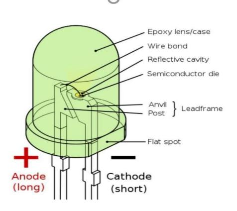
LED Indicator are used as indicating, warning, accidental signals and other signals of instrument circuits in the areas of electric power.
