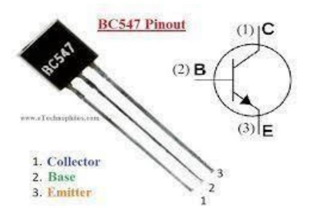
is a NPN transistor hence the collector and emitterwill be left open (Reverse biased) when the base pinisheldatgroundandwillbeclosed(Forwardbiased)whenasignalisprovi ded tobasepin.
