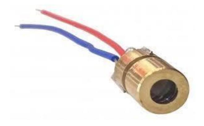
A laser diode is a semiconductor that uses a p-n junction forproducing coherent radiation with the same frequency andphase which is either in the visible or infrared spectrum. It also called an injection laser diode and the technology is similar to that found in LEDs
