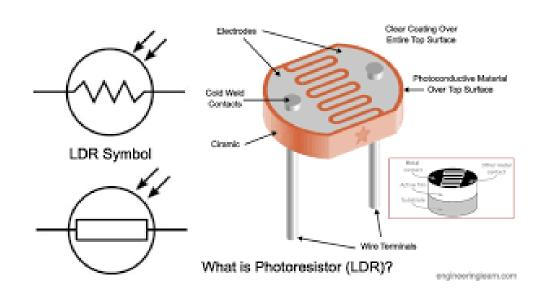
A photoresistor or light dependent resistor isan electronic component that is sensitive to light. When light falls upon it, then the resistancechanges. Values of the resistance of the LDR maychange over many orders of magnitude the value of the resistance falling as the level of light increases.
