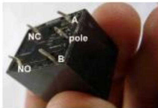
Figure 2.19 Electromagnetic or mechanical relay
